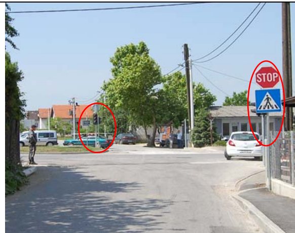
Figure 2.8. Regulation of the traffic with traffic light – bad visibility regarding the signals
