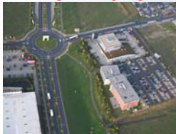
Example for a 2-Lane-Roundabout
